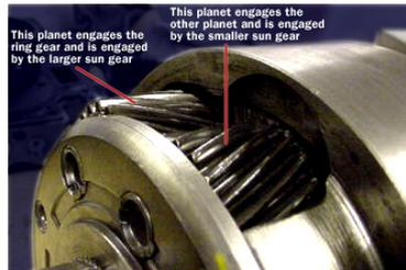
This planet engages the ring gear and is engaged by the larger sun gear
