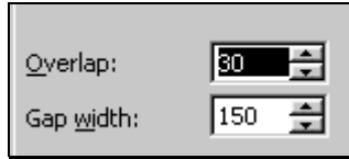
Figure 184: Changing the "Overlap" and "Gap Width" of the 'blocks' that make up one 'stack' of a stacked chart
