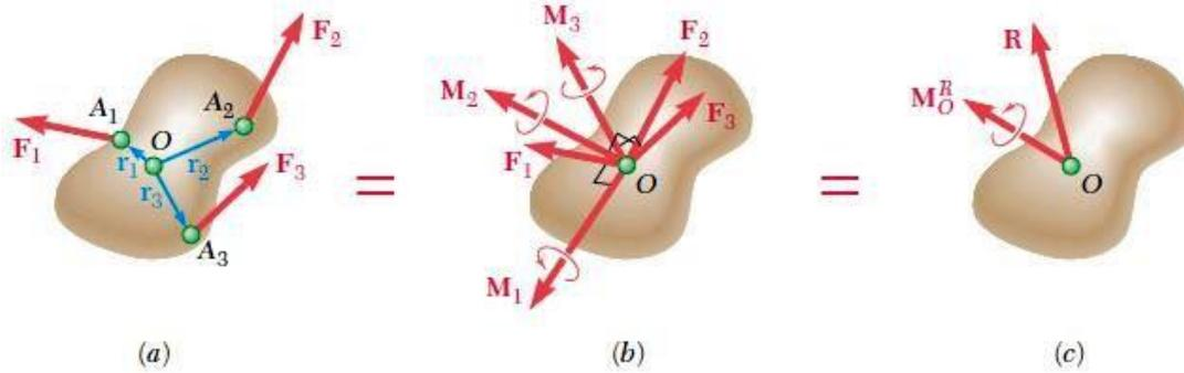
Alors on a :  $\vec{R} = \sum_i \vec{F}_i$  et  $\vec{M}_O^R = \sum_i \vec{M}_{i/O} = \sum_i (\vec{r}_i \wedge \vec{F}_i)$
